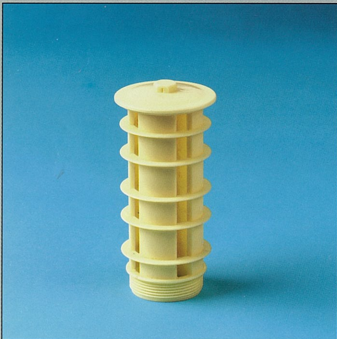
RTA-TB2070 Inlet Baffle 2" npt male thread Open area: 6.35 in 2 Stack diameter: 3.275" Stack height: 5.855" Injection molded polypropylene
