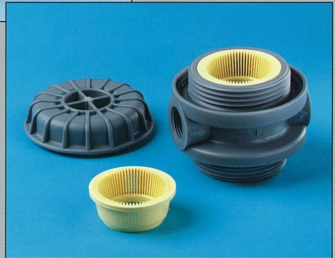
X-KSH-75 Manifold Removable inlet screen Tank access from top cap 3/4" npt external Riser dia.: 1/2", 13/16", 3/4" Center Slot clearance: .0086" Material: Polypropylene
