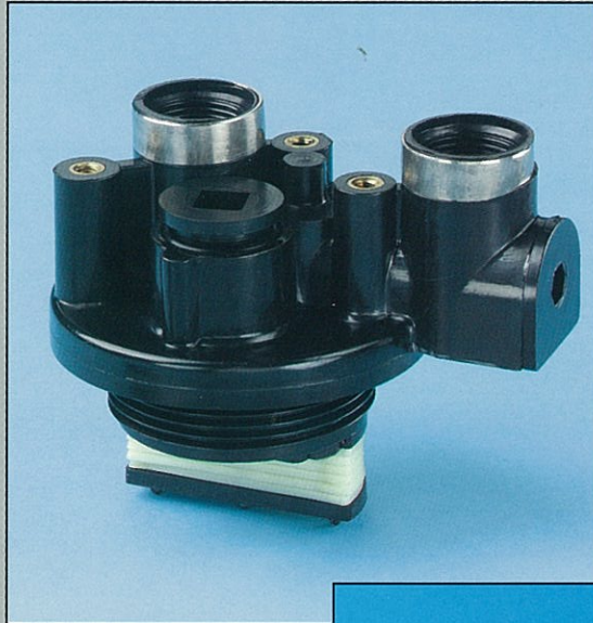
X-PI25-3IS Manifold Inlet screen option 3/4" npt external 3/4" fill port w/cap Stainless inlet ring Portable exchange applications Riser dia.: 1/2", 13/16" Offset Slot clearance: .012" Material: ABS
