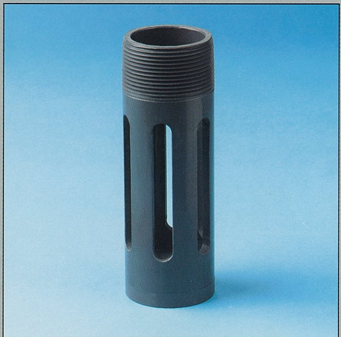
RTA-TB2570 2.5" npt male thread Open area: 17.95 in 2 Stack diameter: 2.875" Stack height: 6.60" Machined PVC
